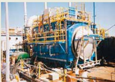
*Gas Phase Chemical Reduction (GPCR) unit used for remediation in Australia.*
