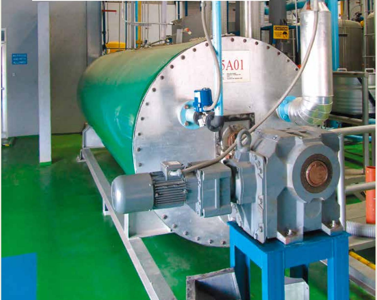
*Sodium Reduction (SR) facility used for destruction of PCB oils in Philippines.*
